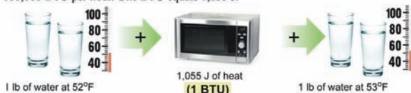
1 BTU raises the temperature of 1 pound of water by 1°F
