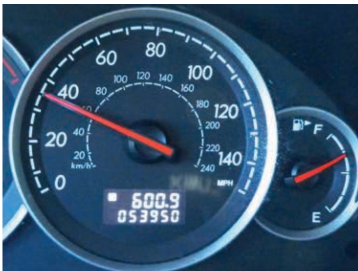
This car speedometer shows speed in miles per hour and in kilometers per hour. Kilometers per hour is the speed unit commonly used in most other countries outside of the United States.
