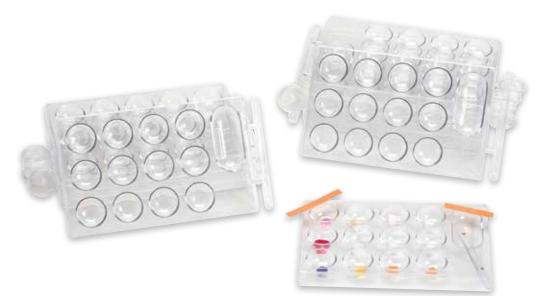
The Lab-Aids<sup>®</sup> Chemplate<sup>®</sup> is a clear plastic tray about the size of an index card. It has changed thousands of science teachers' ideas of how to conduct labs. Using the inexpensive Chemplate<sup>®</sup> eliminates the need for glassware and provides a semi-micro environment for conducting many experiments.
